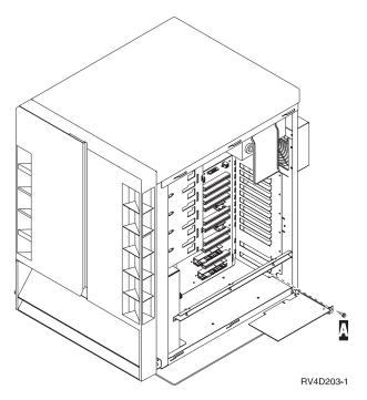
Figure 6. Install Adapter Card
